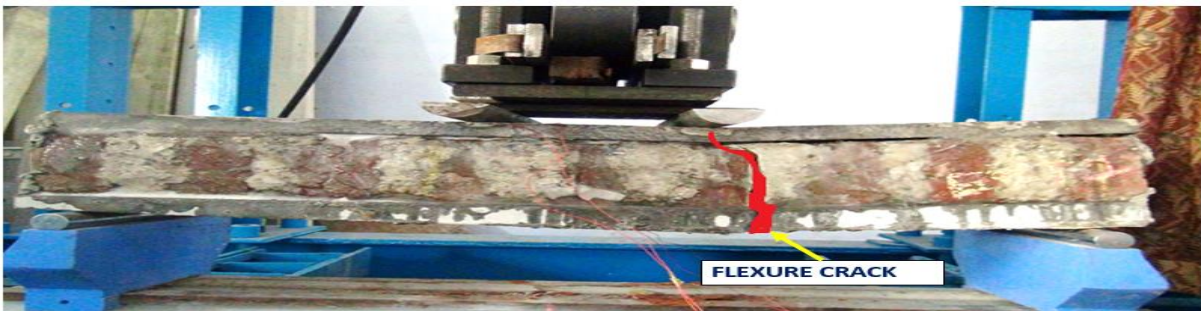
Figure 7 Failure of sandwich beam with epoxy as bonding agent
